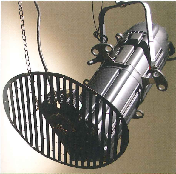
FIGURE 17. THIS PROFILE IS FITTED WITH AN ANIMATION DISC, WHICH, AS THE NAME SUGGESTS, IS USED TO ADD AN IMPRESSION OF MOVEMENT IN THE BEAM. USUALLY USED IN CONJUNCTION WITH A GOBO, ANIMATION DISCS CAN HELP TO IMITATE THE LIGHT REFLECTED FROM WATER, OR LIGHT FROM A FIRE, OR APPIA'S LIGHT FILTERED THROUGH A FOREST CANOPY.
